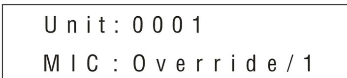
The information displayed on the home screen is shown in the figure above, including unit (indicating the number of conference microphone units connected to the system from "0001" to "4000"), conference mode (Override, Voice, Open, or Apply), and the maximum number of speeches (1, 2, 4, or 6).
