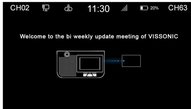
Sign-in by NFC card allows accurate identification of user image, name, position, etc. (Add user details in the system management software. Refer to 5.2 - 5.3.)
