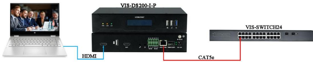
Figure 2.7.2 External video source access to switch via VIS-DS200-I-P
