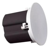
This model of POE speaker is installed on the ceiling, built-in POE amplifier, with gain, equalization, pressure limit, noise gate, mute control adjustment. The speaker only needs to connect a network cable to realize audio, power supply, DSP configuration and real-time signal control, compatible with 802.3af, compatible with 802.3at, natural convection heat dissipation. Ceiling speakers are widely used at Office buildings, hotels, and shopping malls are public places that use ceiling speakers.
