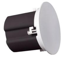
This model of POE speaker is installed on the ceiling, built-in POE amplifier, with gain, equalization, pressure limit, noise gate, mute control adjustment. The speaker only needs to connect a network cable to realize audio, power supply, DSP configuration and real-time signal control, compatible with 802.3af, compatible with 802.3at, natural convection heat dissipation. Ceiling speakers are widely used at Office buildings, hotels, and shopping malls are public places that use ceiling speakers.
