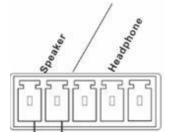
2x 5 pin phoenix connector for speaker and headphone Headphone Output independence:  $16 \Omega$ Speaker output independence:  $8\Omega$ Frequency response:  $20 \sim 15000$ hz
