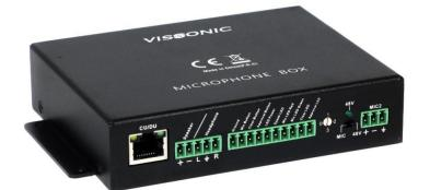
The VIS-AIB microphone interface box is designed to support VISSONIC conference microphone remotely installed under the table or armrest solution. With the phoenix connectors on both sides of the box, it can connect Dynamic mic/Boundary Condenser mic input, buttons and speakers on plate to control the conference unit etc. By the RJ45 port it can easily connect into existing VISSONIC conference microphone family to integrated into one part seamlessly.
