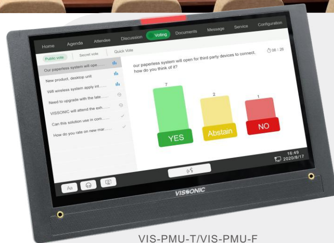
VIS-PMU-T/VIS-PMU-F Desktop/Embedded 11.6" paperless conference terminal
